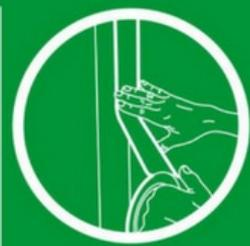
4. For jointing, overlap the VCL membrane by approx. 10cm and seal overlap with Visqueen Single sided Vapour Tape.
