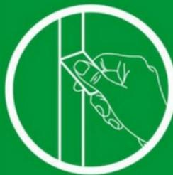
2. Carefully peel off release liner of the Visqueen Double Sided Vapour Tape.
