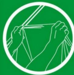
3. Apply the Visqueen Vapour Control Layer membrane to the frame and use a seam roller to press on each strut to ensure a good bond.
