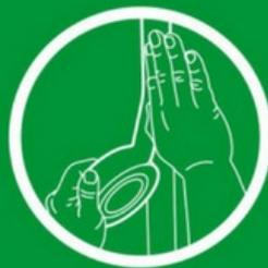
1. Apply Visqueen Double Sided Vapour Tape to the timber (or metal) studs, head and sole plate.
