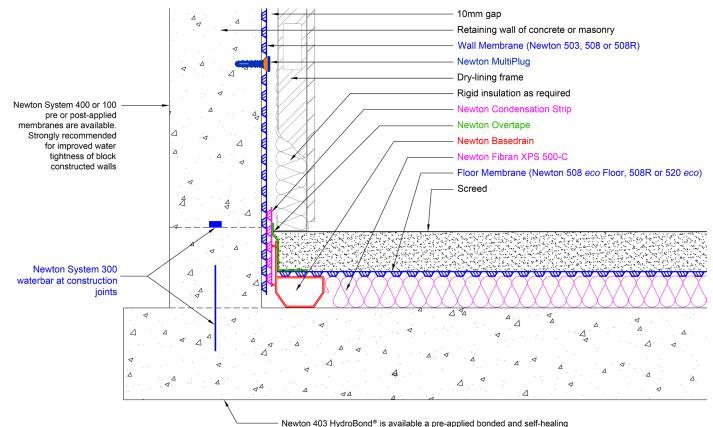
Newton 403 HydroBond<sup>®</sup> is available a pre-applied bonded and self-healing sheet membrane to further waterproof the structure.
