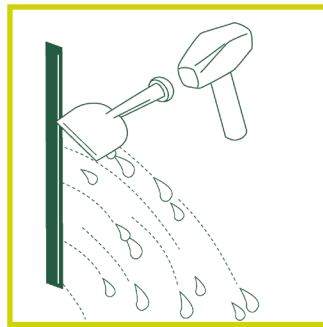
Open up crack to remove any loose material and to provide a key for the WATERSTOP.
