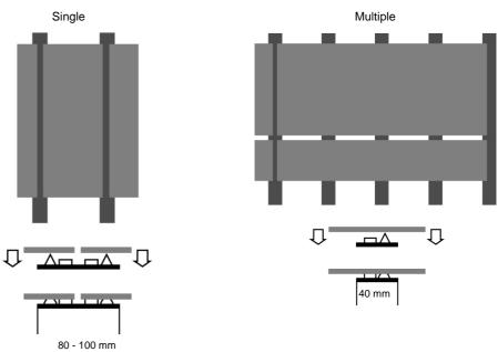
Required width of substructure battens for the use of the SikaTack®-Panel System.
